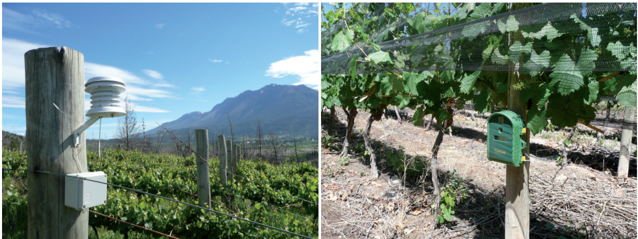
Figure 3 - Temperature sensor (a) and Plant Cam (b).
